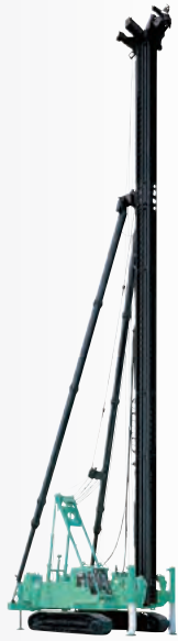
Pile Driving Rig
