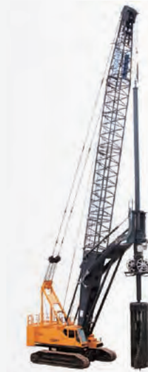
Earth Drilling Rig
