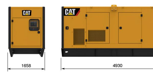
Approximate weight of enclosure package: 4780 kg (10,538 lb). Exact weight is dependent on options. Enclosure weight includes: sound attenuated enclosure, exhaust system, base and generator set. Generator set enclosure also available in white. (Caterpillar yellow is standard colour)
